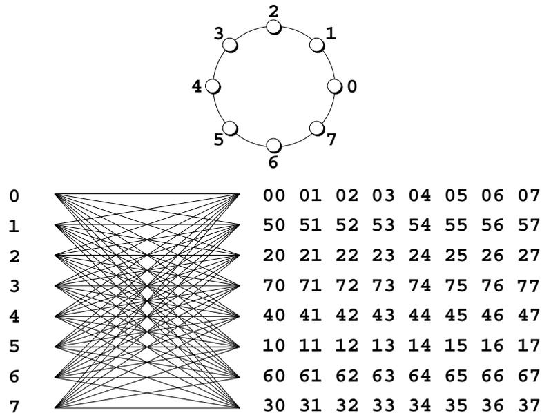
Figure 1.2. 8-State 8-PSK Space-Time Trellis Code with Two Transmit Antennas and a Spectral Efficiency of 3 bits/sec/Hz
