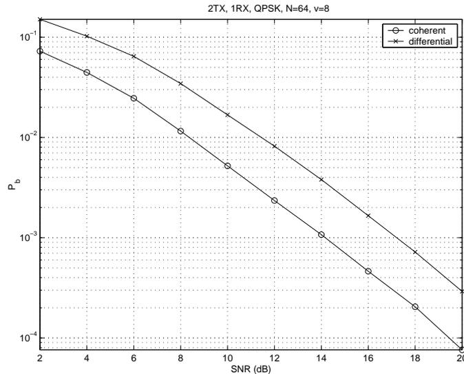
Figure 1.12. Performance Comparison Between Coherent and Differential OFDM-STBC with 2 TX, 1RX, QPSK Modulation, FFT Size of 64,  $\nu = 8$
