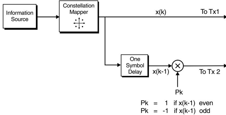
Figure 1.3. Equivalent Encoder Model for 8-State 8-PSK Space-Time Trellis Code with Two Transmit Antennas
