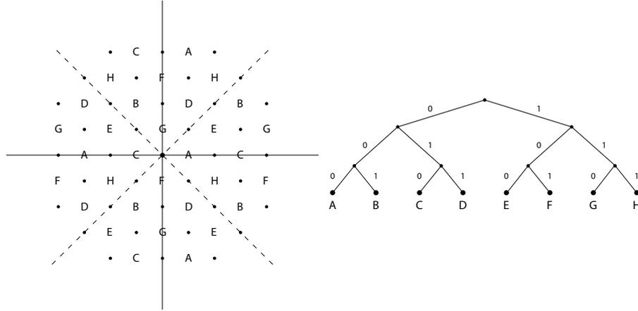
Figure 1.8. A Binary Partition of a 32-Point QAM Constellation
