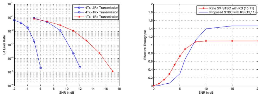
Figure 1.5. Left Figure Compares Quaternionic Code with Single-Antenna Case for WiMAX. Right Figure Compares Effective Throughput of Quaternionic Code with Octonion in a Quasi-Static Channel
