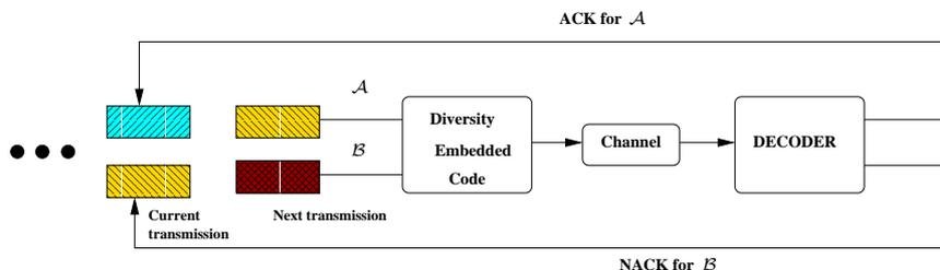
Figure 1.15. ARQ mechanism for diversity embedded codes using prioritized scheduling.
