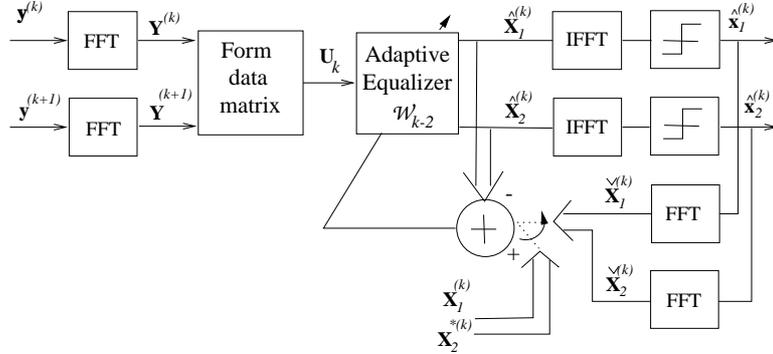
Figure 1.11. Block Diagram of Adaptive FDE-STBC Joint Equalizer/Decoder
