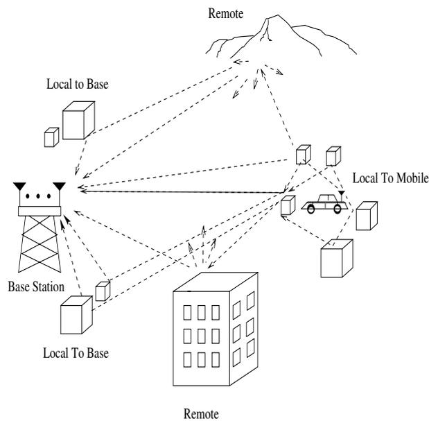
Figure 1.1. Radio Propagation Environment
