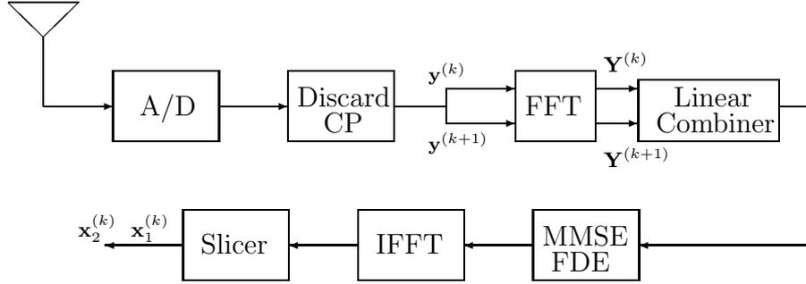
Figure 1.10. FDE-STBC Receiver Block Diagram
