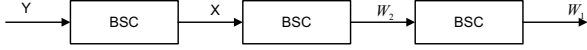
Figure 2: The optimal forward test channel in Region I-B. The crossover probability for the BSC between X and W_2 is D_2 , while the crossover probability \eta for the BSC between W_2 and W_1 is such that D_2 * \eta = D_1 .
