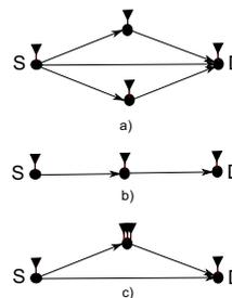
Fig. 1. a) Single relay network. b) Line relay network. c) The relay channel with multiple antennas
