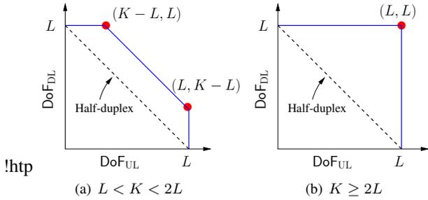
Fig. 2. The DoF region in full-duplex network with  $L$  antenna base-station and  $K$  single antenna mobile-station
