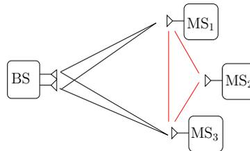
Fig. 1. Network with 2 antenna base-station and 3 single antenna mobile stations. The inter-node interference is between the mobile stations is also highlighted.
