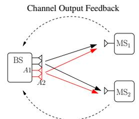
Fig. 5.  $(2, 2)$  full-duplex network w/o uplink messages is enhanced to a  $(4, 2)$  half-duplex network with channel output feedback
