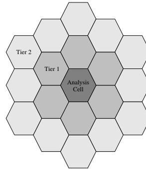
**Figure 2: Cellular Simulation Diagram.** The Analysis Cell base station forms a beam with the Analysis Cell user as the objective and Tier 1 cell users as constraints. The Tier 1 cell base stations form beams with their desired user as the objective and adjacent users from Analysis Cell, Tier 1 cells, and Tier 2 cells as constraints. No base stations are present in Tier 2-only users which form constraints for Tier 1 cells.
