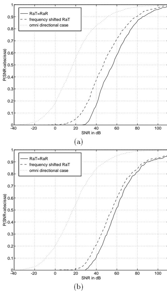
**Figure 3:** (a) SINR cdf for angle spread of  $10^\circ$ , success rate=71%. (b) SINR cdf for angle spread of  $30^\circ$ , success rate=46%.
