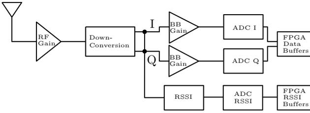
Figure 5: Radio board receiver path
