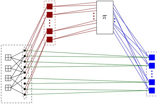
Figure 2: LDPC-based joint decoder for QMF
