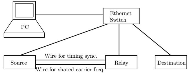
Figure 3: Node and host PC configuration
