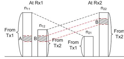
Fig. 1. Two-user deterministic interference channel. Levels A and B interfere at the 1<sup>st</sup> receiver, and cannot be fully active simultaneously.
