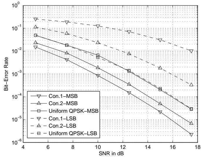
Fig. 3. Layer A BER Performance for Example 1 with Hierarchical and Uniform QPSK Constellations
